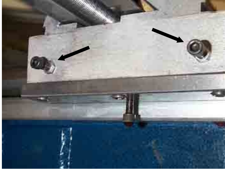
Fig. A5.2 - Brass Gib adjustment screws for the Saddle.
