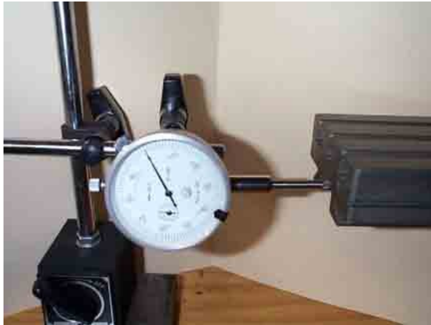
Fig. A3 - Measuring the X-axis Backlash.
