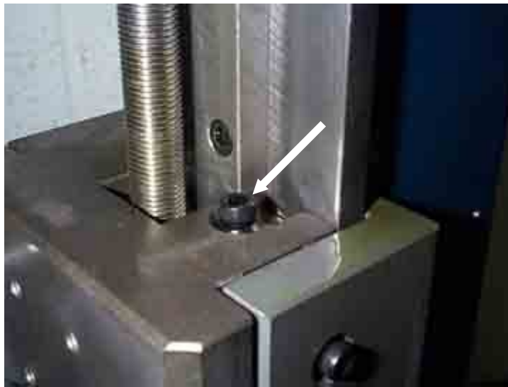
Fig. A5.1 - Box Way Brass Gib top adjustment screw.
