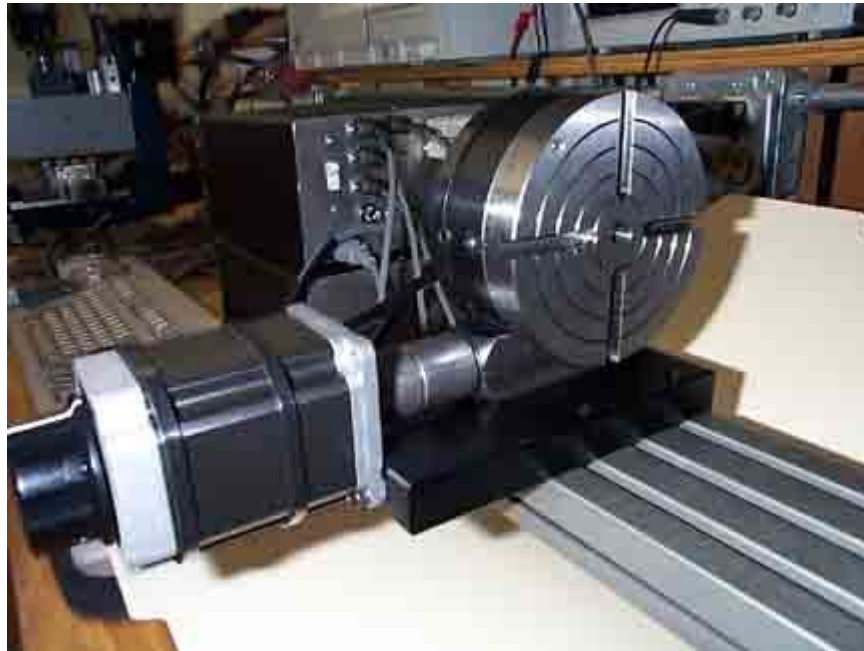
Fig. 22 - Standard mounting position of the 4 th Axis Rotary Table.
