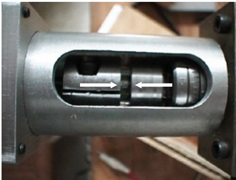
Fig. 3a - Setting the coupling Gap.
