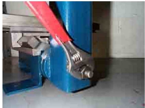
Fig. 4 - Quick squaring of Spindle to Table.
