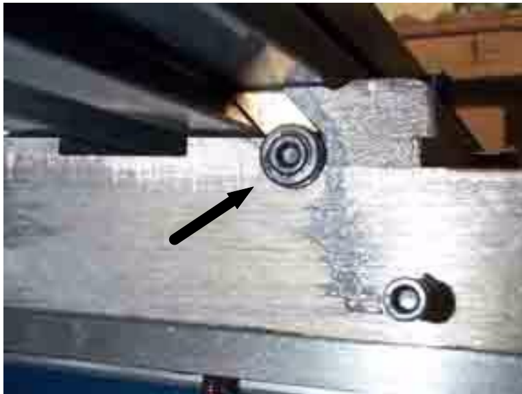
Fig. A5.3 - Tapered Brass Gib adjustment screws for Table.
