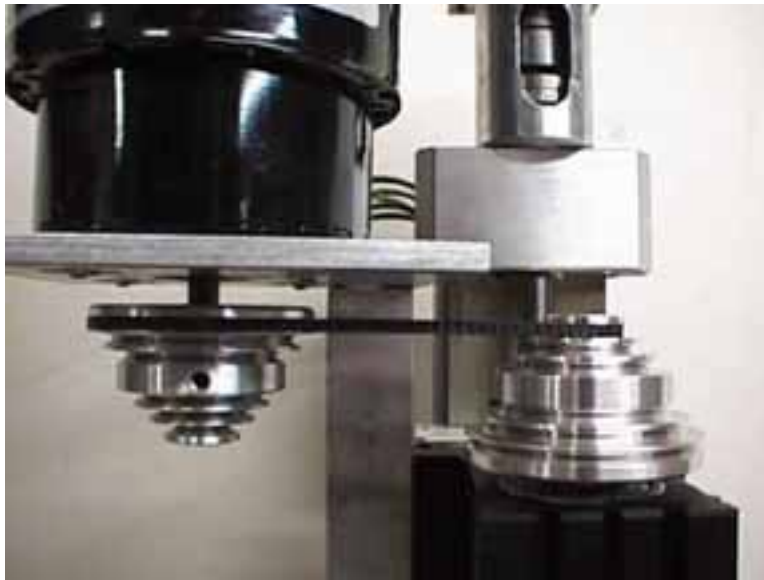
Fig. 9 - Spindle set to top speed position.
